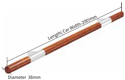
H06-00 (Wooden Round Handrail) Black Walnut Round Handrail + Mirror ST.ST. Bracket
